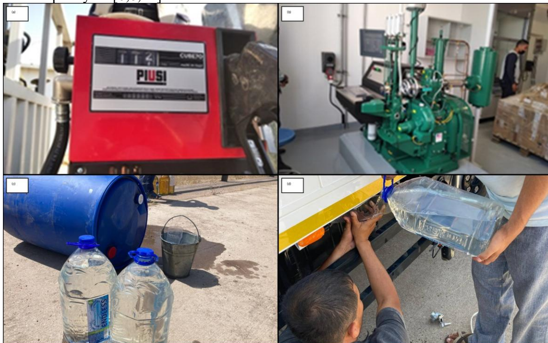
Figure 1. Experimental documentation of the GTL tests: (a) PIUSI digital fuel-flow meter; (b) laboratory engine test stand; (c) GTL fuel samples and storage barrels; (d) refuelling of the ISUZU NQR71PL test vehicle.
